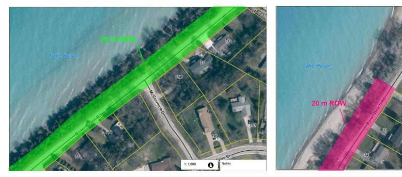
The roadway is not centered in the ROW and the protected shoreline already occupies a variable portion of the existing 20 metre right-of-way
