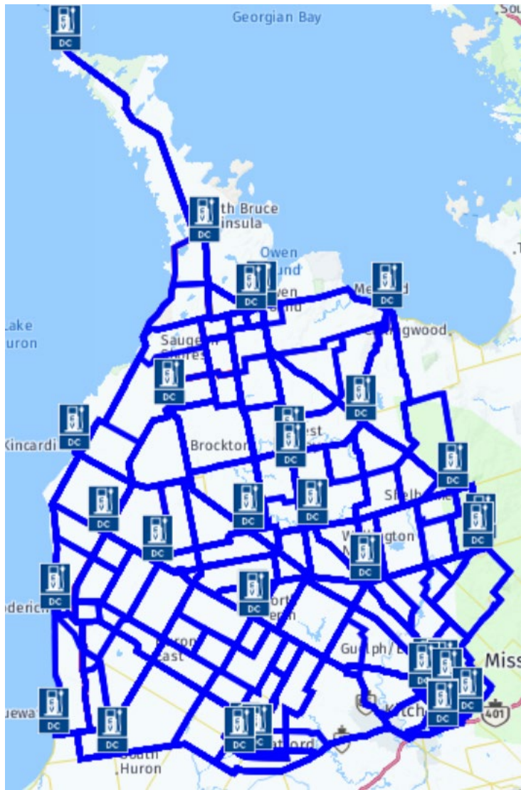
Figure 14. Regional EV charging network (including existing stations) after installation of Baseline/Phase 1 (12) Level 3 EV charging stations. Blue lines indicate which routes are travelable by an EV without any range limitations.
