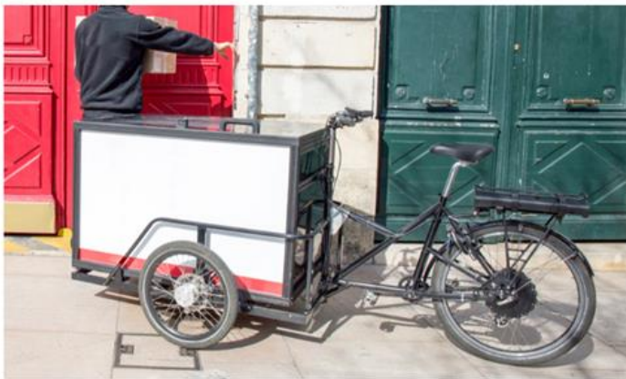
Tricycle cargo e-bike design with enclosed cargo box at the back
