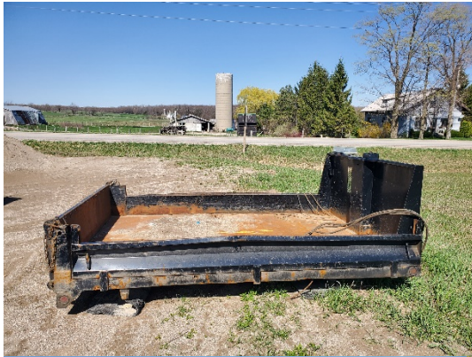
Dump Box with hydraulic cylinder
