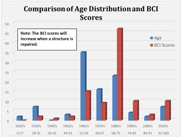
Figure was created to see if the BCI scores for the bridges deteriorated linearly from 100 to 40 over; over 80 years as suggested.
