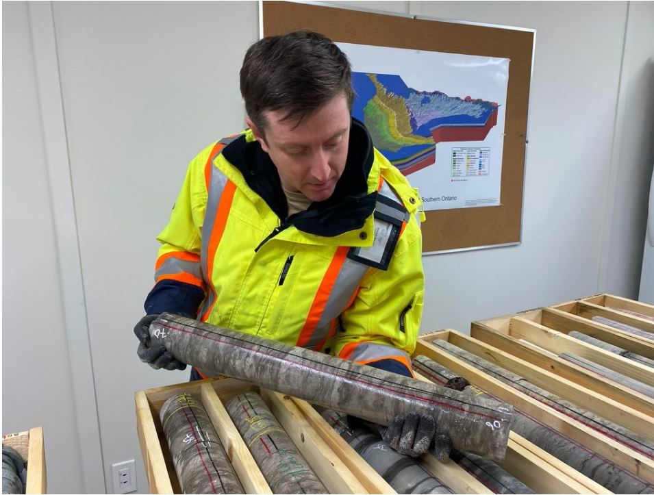
Figure 3.5: Photo of Cobourg Formation core sample from the NWMO's first borehole at the South Bruce Site.
