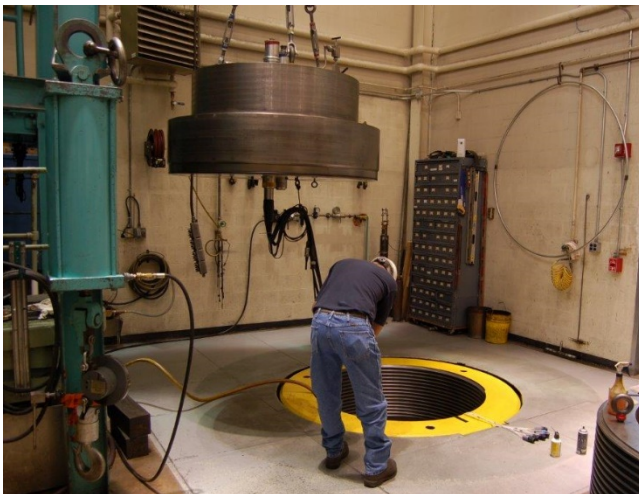
Figure 7.5: Prototype Used Fuel Container subjected to external pressure equivalent to almost 6 km underwater. (Left) Test chamber lid being lowered into place; (Right) Container removed after testing; fully intact – no containment failure.
